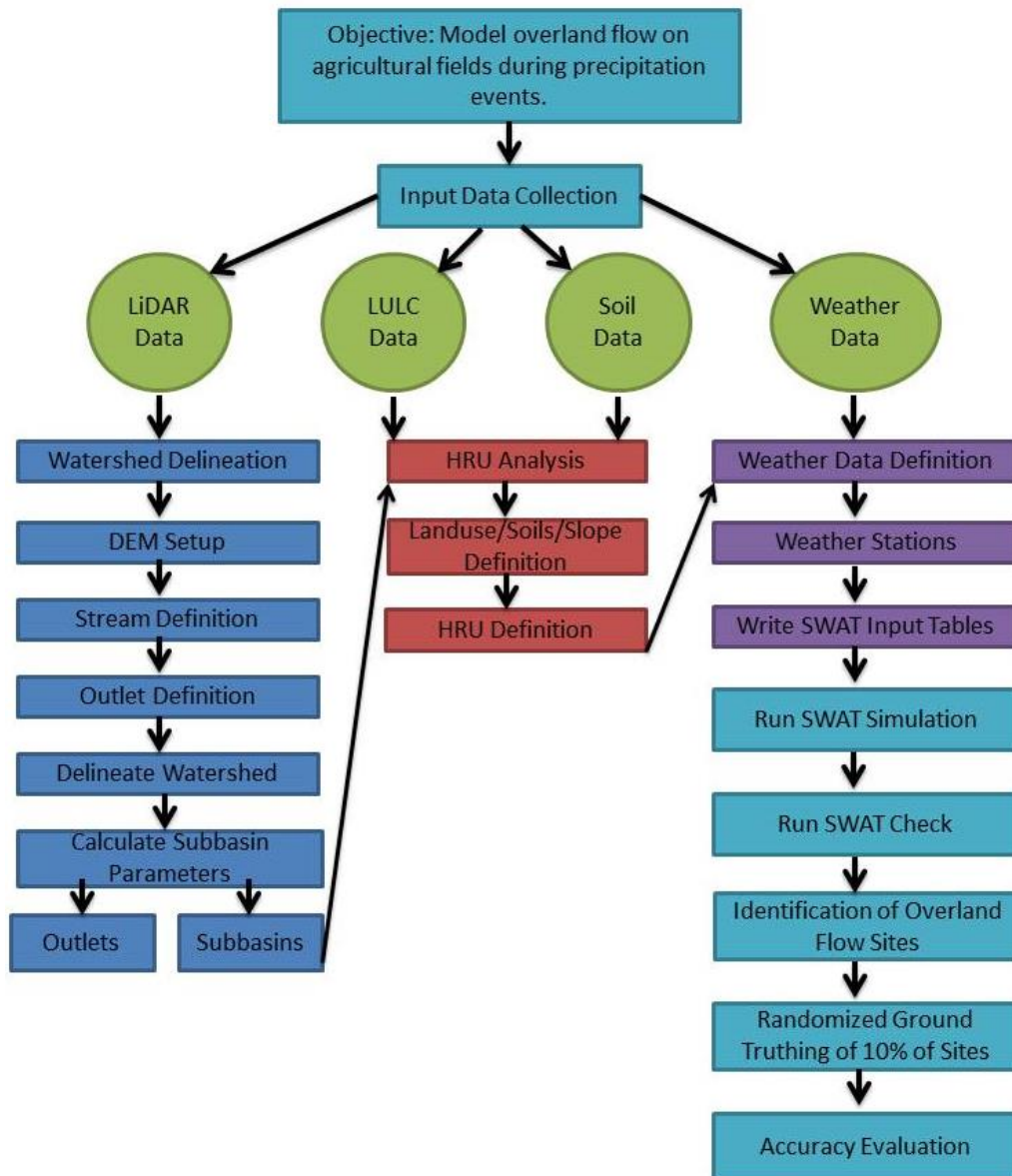
Figure 3. Schematic model of the Soil and Water Assessment Tool and accompanying user-defined methodology that described the three main workflows that the model required before the simulation was produced. Those workflows were: Watershed Delineation (dark blue), HRU Analysis (red), and Weather Data Definition (purple/teal, Duy Liem, 2012). Abbreviations legend: light detection and ranging (LiDAR), land use and
